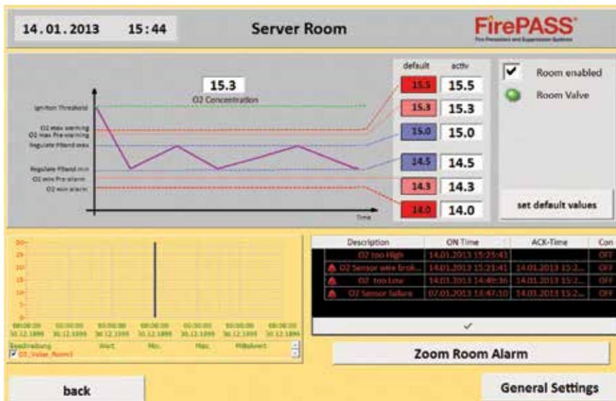
Example: The “room info screen” shows all relevant system parameters including actual and past oxygen values.
